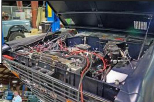
This under construction Bronco is be fitted with modern fuel injection.
