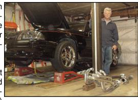
remove factory caytalic converter air supply system hardware 6) disconnect plug wires and remove spark plugs 7) Remove existing shorty headers (which by the way just easily lifted out) 8) Remove strut tower and under car sub frame braces 9) Remove starter.
